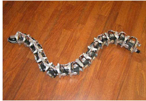
Fig. 2 – All-Terrain Multi-Sensor Snake Robot
