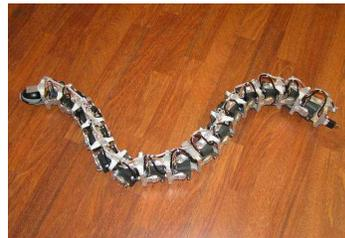
Fig. 2 – All-Terrain Multi-Sensor Snake Robot
